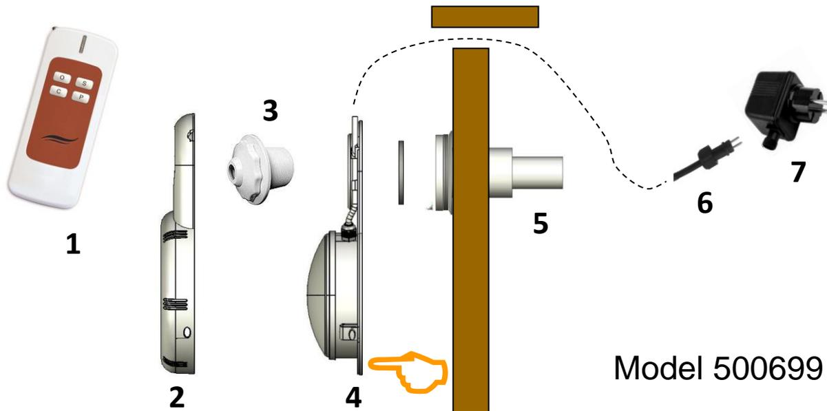
Caution: the minimum distance between the swimming-pool and the provided transformer must be 3,50 m in use
