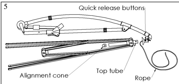
6. Ensuring the canopy's top side is out, fit the center hole of the canopy over the top tube of the cage assembly.
