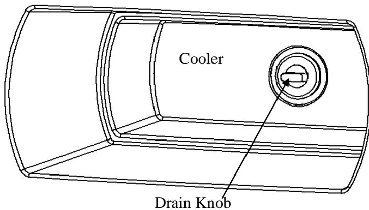
To drain the melt water from your cooler, turn the drain knob a couple of turns counterclockwise. Melt water will exit through the small hose located on the umbrella side, low by the lifter. This hose can be gently pulled out to help pour into a container. When done simply push the hose back into the cabinet until it hits the hose stop.
