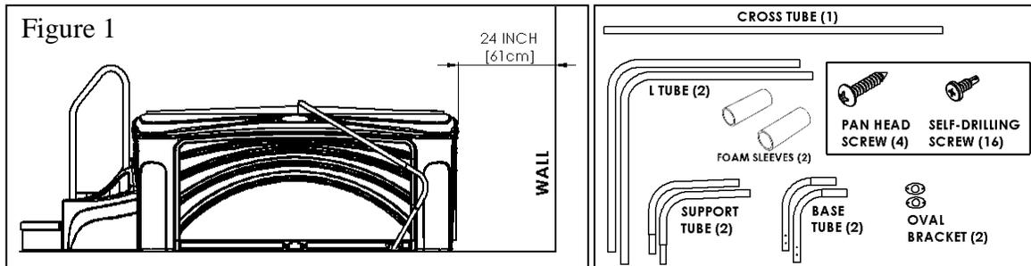
1. Place your spa cover in its proper position on the spa shown in Figure 1. The cover hinge will be parallel to the lower lifter holes shown in Figure 2.
